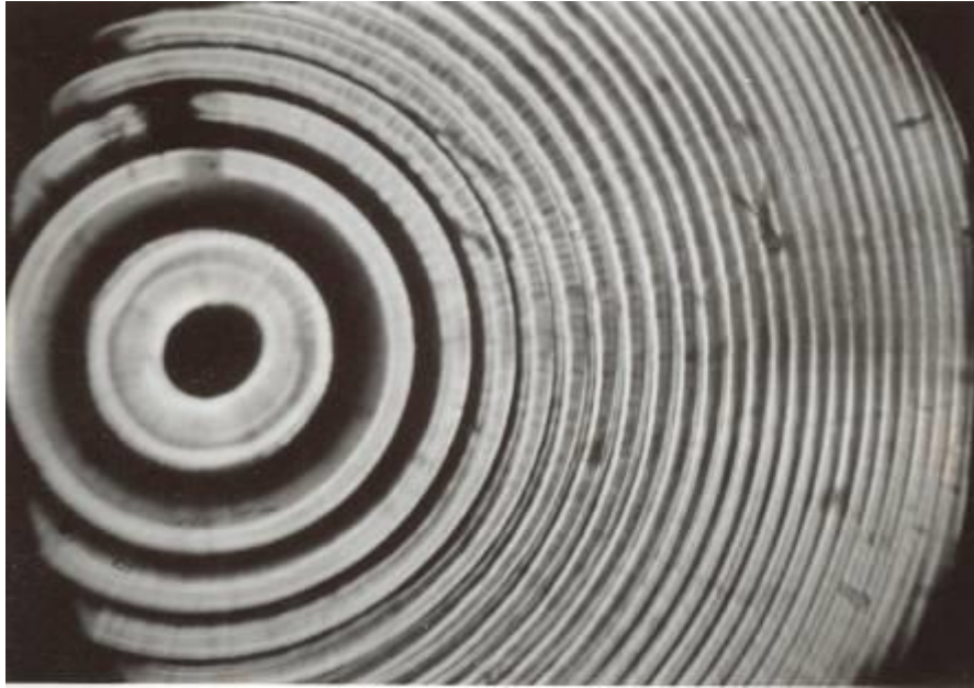
Microphoto of cross section of produced preform
